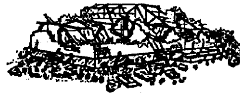
DG 5 - Destruction: total or near total collapse
