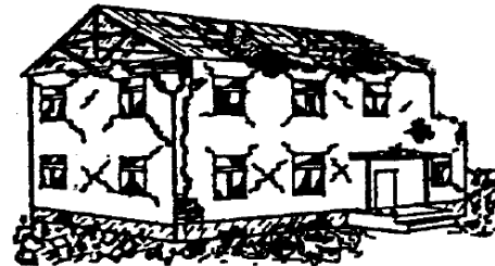
DG 4 – Very heavy damage: serious failure of walls
