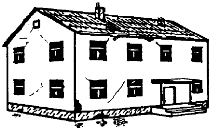
DG 2 – Moderate damage: cracks in walls, partial collapse of chimneys
